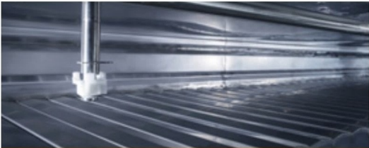
Clean-in-Place (CIP) Upgrade for Existing Freezers
